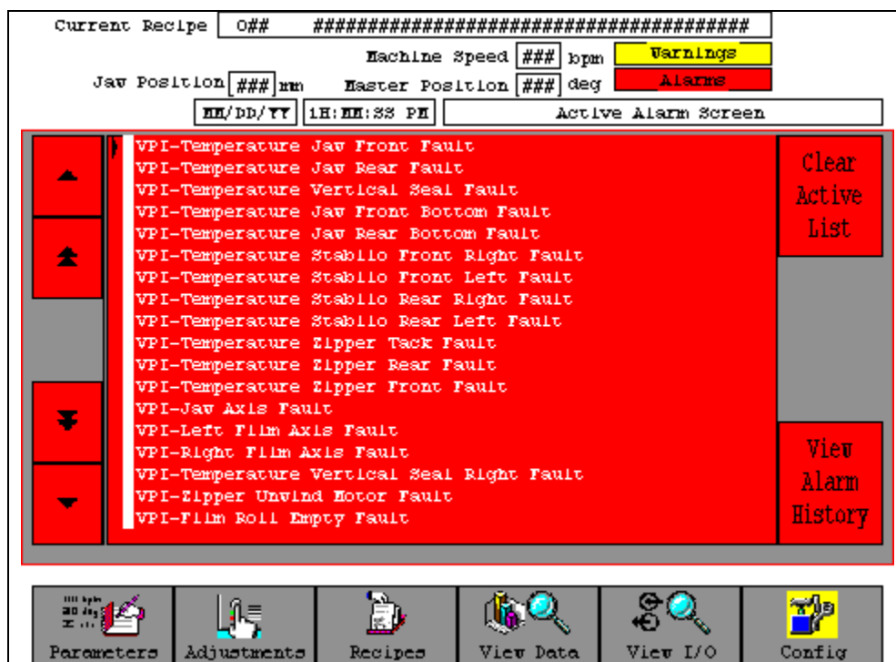
Figure 5.25 Shows the Alarms screen.
