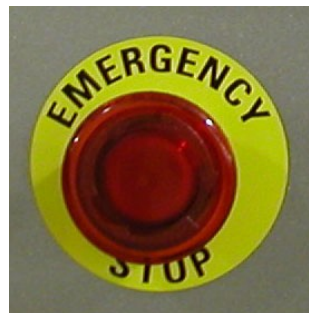
Figure 5.30 Shows the EMERGENCY STOP push-button.
