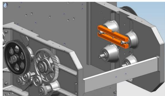
*alignment tool for cross sealing station in ROVEMA form, fill and seal machine*
